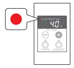
Check ignition, combustion and extinction of the unit by the "In Use" indicator light of the controllers.
