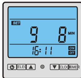
Parameter 9 Exit defrost backup mode Range: 1 to 12 min. Default: 8 min Adjustable by technicians
