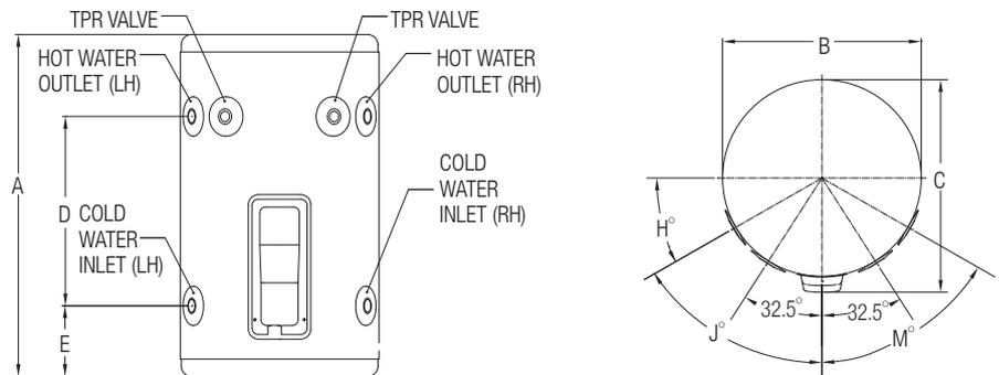
50L models have left and right hand (dual handed - DH) cold water connections, hot water connections, and T&PR valve fittings.
