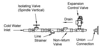
**Note:** a combined isolating valve/non-return valve/line strainer may be used. Expansion control valve only required where local regulations demand.
