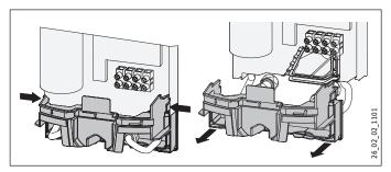
► Remove the back panel by pressing the two locking hooks and pulling the lower part of the back panel forwards.
